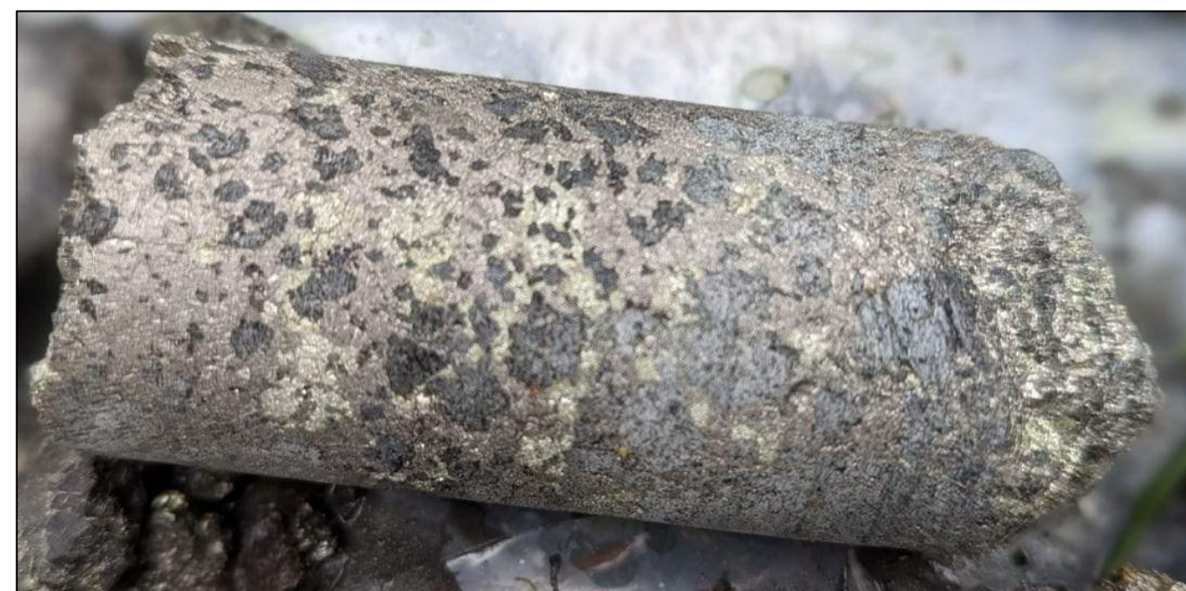
Closeup of mineralization in backpack core from the Taureau showing with semi-massive sulphide (pyrrhotite and chalcopyrite) mineralization.
