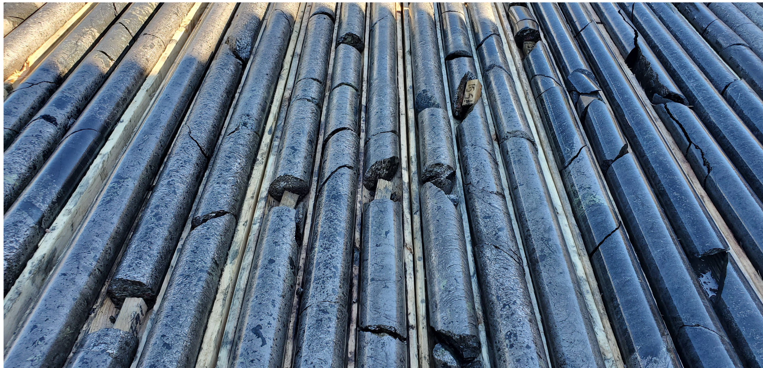
Magmatic Nickel Sulphide Mineralization from BDF22-002
